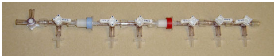
Figure 2 Quick-fit processing units (left to right, V1-2, QMA, V3-4, C18, V5-7; male luer slips on V2 and V4 are press-fitted to the structural support, while all others drain into collection tubes).
