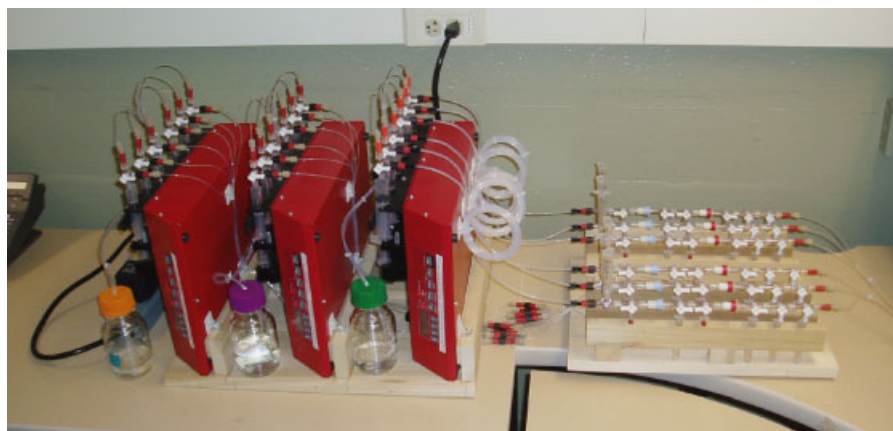
Figure 3 Full layout of the multi-sample tandem SepPak (QMA/C-18) processor. Pumps A-C (right to left) are shown. The sample loops (six) on Pump A are directly connected to the processing lanes (six) through V1 in each lane. Each processor lane receives inputs from all three pumps.
